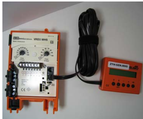
Lead connected to a VRD3.MHS
