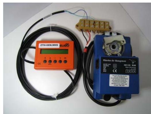
Lead connected to a NMV-D2
