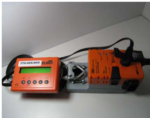
Lead connected to a NMV-D3-MP.MHS
