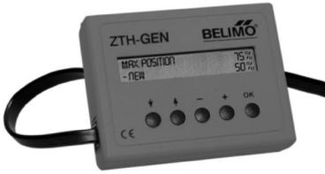
Service-Tool for parameterisable and communicative Belimo actuators and VAV controllers. Local connection via service socket on the device or remote control via MP/PP connection.
