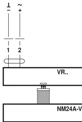
The ready-to-connect operating unit is connected to the VR.. controller with the 3-pin plug.
