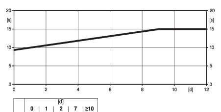
[d] = Electricity interruption in days[s] = Pre-charging time in secondsPF[s] = Bridging time
