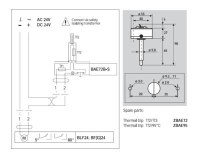
If any of the internal thermal fuses blow in the BAE72-S, it is possible just to replace the fuse part with the service replacement fuse section ZBAE72.
