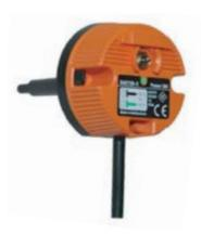
The BAE72-S is a duct mounted thermal fuse with local test switch, this safety fuse comes pre-wired to the Belimo BF-T or BLF-T range of fire/smoke spring return damper actuators (Note:- some BAE units are fitted with a green indication LED).
